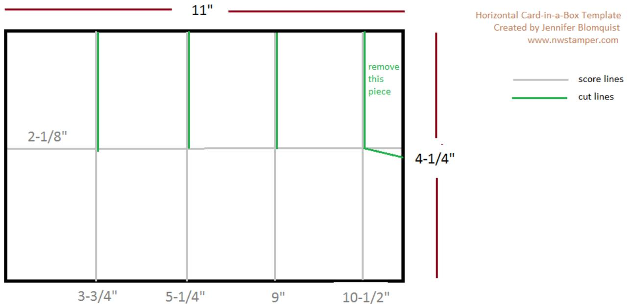
3. Cut as shown in the diagram above and then adhere the 1/2" x 2-1/8" tab to the inside of your box with Sticky Strip.
